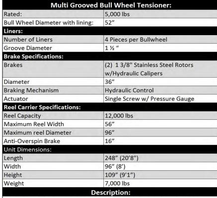
The OLT52B Bull Wheel Tensioner is designed to install right hand single lay conductor.
