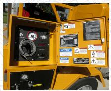
The TSE Model UP-85BD Underground cable puller provides infinite speed control and precise tension and distance monitoring. The 8" bullwheels are powered by a hydrostatic drive with a variable displacement axial piston pump and a two speed hydraulic motor. The cable payout is on demand with the bullwheel drive system feeding the pulling rope when any load in excess of 1 lb. is placed on the cable.
